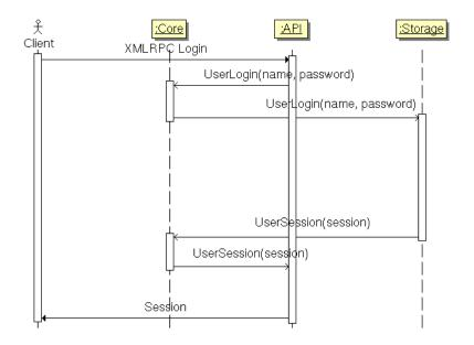
Figure 3.3: Log in sequence diagram
