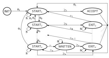
Fig. 6. Automaton detecting fully initialized arrays.
