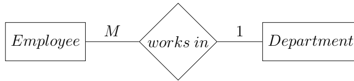
Figure B.4: An ER-model where a RELATIONAL_COLLECTION_PART with 1:M mapping can be used.
