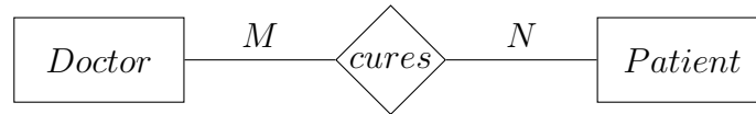
Figure B.5: An ER-model where a RELATIONAL_COLLECTION_PART with M:N mapping can be used.
