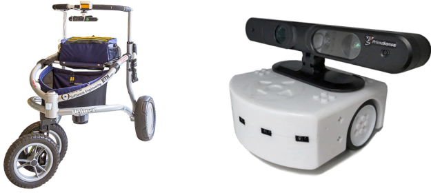
(a) SmartWalker – the robot for ambient assisted living (AAL) with PrimeSense RGBD sensor (b) Educational robot Thymio-II
