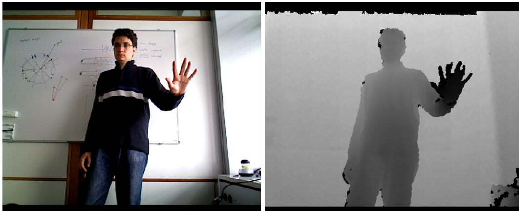
Figure 2.3: RGB and depth image of the Primesense camera
