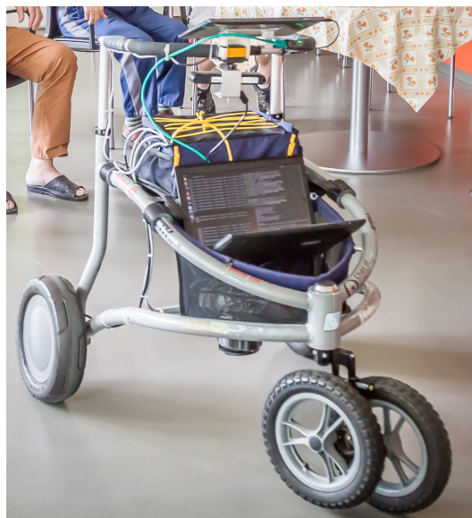
Figure 2.2: The SmartWalker with an additional Laptop for face and gesture recognition.
