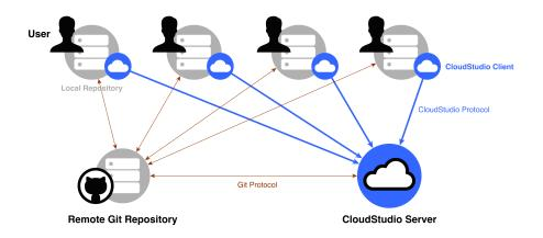
Fig. 2.1: Typical CloudStudio setup for a single repository
