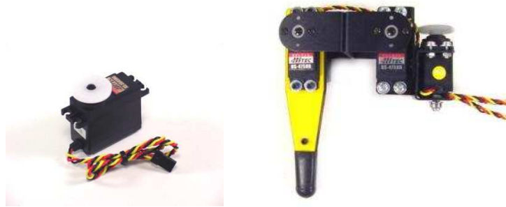
Figure 33: Servo motor and its placement on the leg
