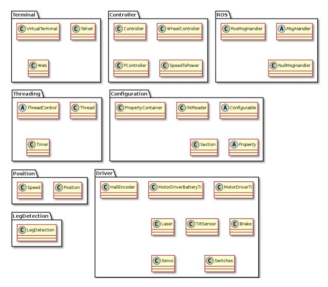
Figure 10: UML diagram of all packages and important classes
