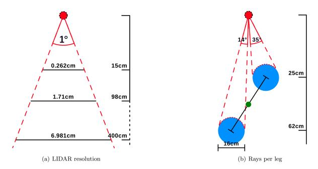
Figure 20: XV-11 LiDAR capabilities
