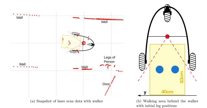
Figure 22: Filter data points outside of the walking area
