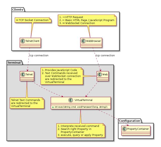
Figure 12: UML diagram of the Terminal package
