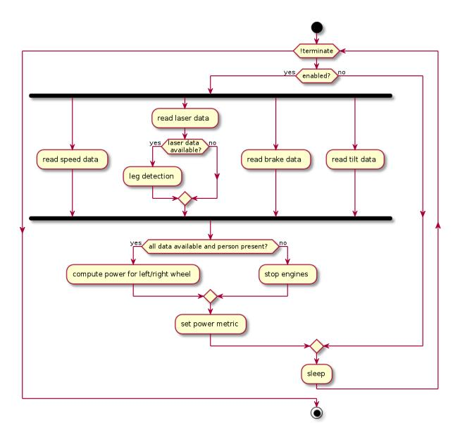
Figure 30: STP control loop
