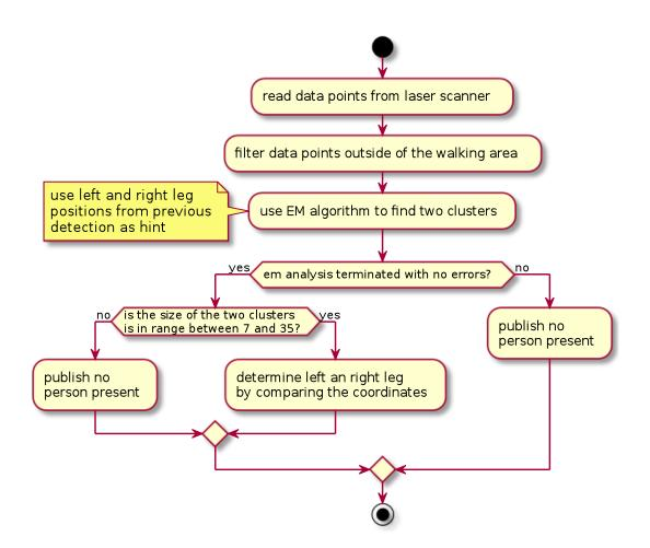
Figure 21: Leg detection algorithm
