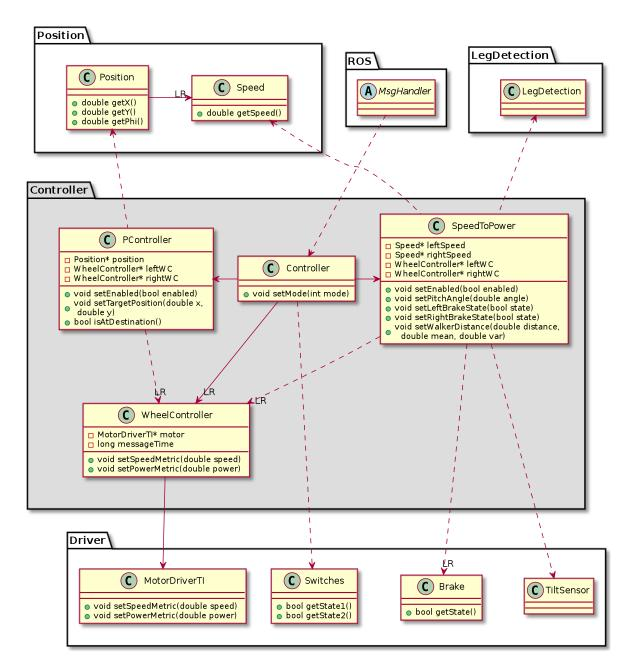
Figure 27: UML diagram of the Controller package
