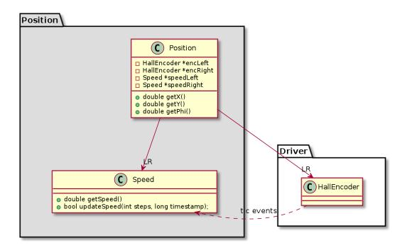
Figure 17: UML diagram of the Position package
