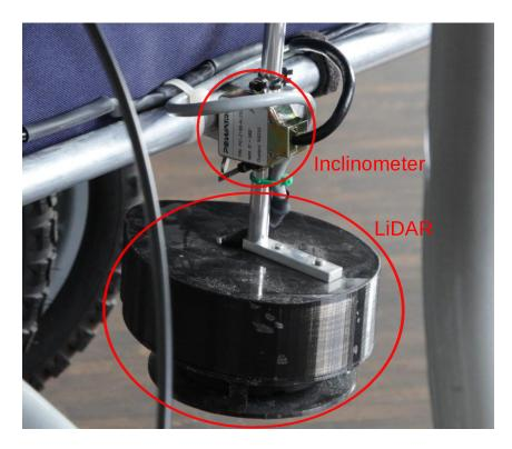
Figure 6: LiDAR of the SMARTWALKER
