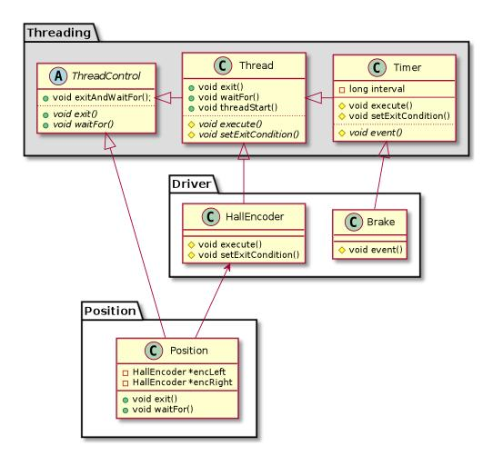
Figure 18: UML diagram of the Threading package
