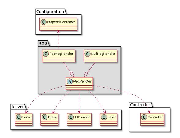
Figure 16: UML diagram of the ROS package
