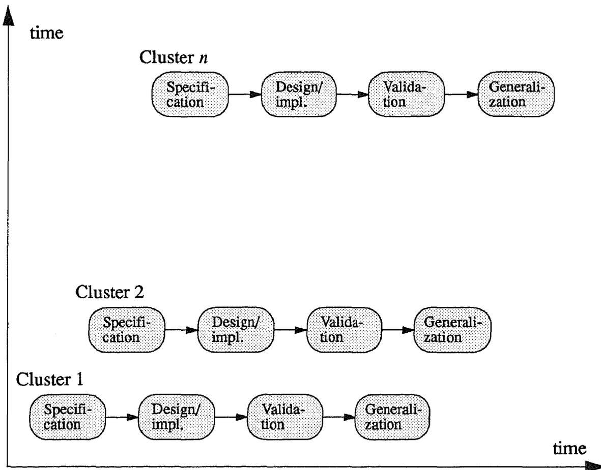
Figure 2.6 The cluster model of the software lifecycle.
