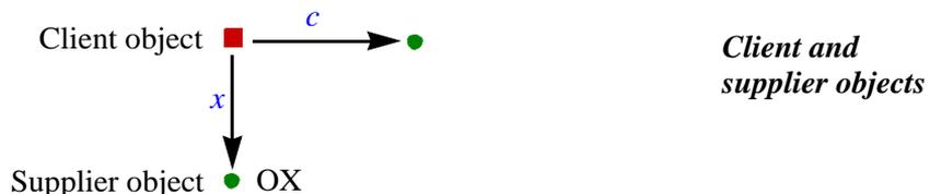
The figure (using the precise conventions of “alias diagrams” introduced in [16] for presenting properties of object structures) also shows a field of the client object, corresponding to an attribute  $c$ , which can be used as an actual argument to the call (part of the list  $l$ ).
